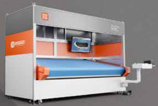
PN-3216-E 数控皮革排版机 CNC leather nesting machine
